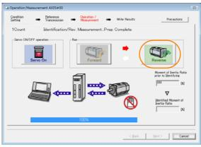
The Servomotor shaft will rotate in the reverse direction and the measurement will start. After the measurement and data transfer have been completed, the **Forward** Button will be displayed in color.
